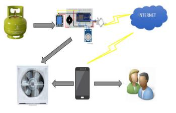
Figure 1. Architecture of a Gas Leak Detection System
